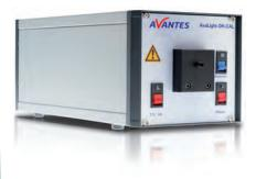
For calibrations in the ultraviolet and visible range (200-1099 nm), the AvaLight-DH-CAL is the best solution. This source can be used with all AvaSpec spectrometers to calibrate for absolute spectral intensity. It is supplied with a built-in diffuser, a cosine corrector (CC-VIS/NIR) with SMA adapter and the calibration files in ASCII format.
